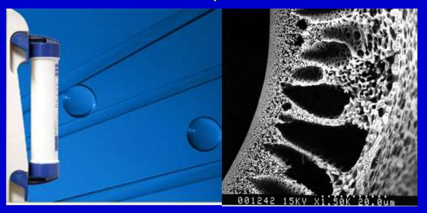
Ultrafilters Remove Bacterial Products by Size Exclusion and Adsorption
